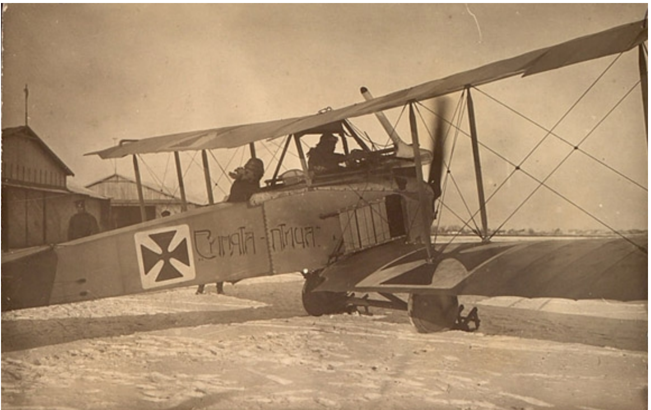
LVG B.II (Otto) from the Aviation Squadron of the Kingdom of Bulgaria. The plane was actively used in the offensive operation against Serbia. What's noticeable is the unusual placement of the identification marks on the wings.
